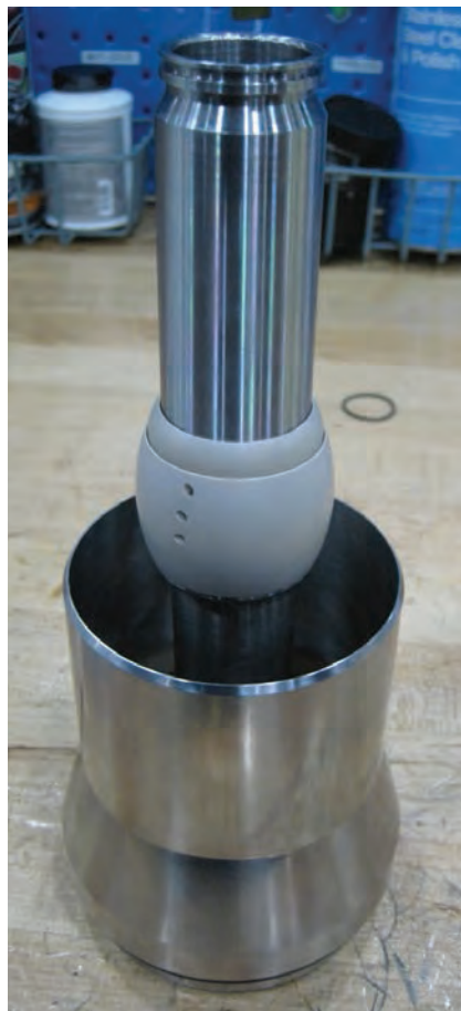
4. Nozzle and lock ring slides over spindle.
