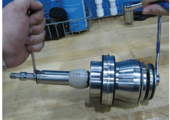
14. Tighten. Use a 13mm and 16mm wrench. Torque 20Nm.
