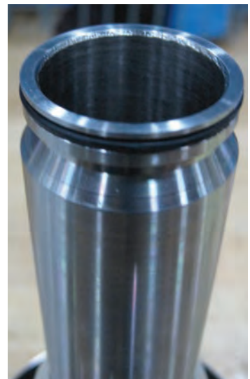
5. Mount o-ring on upper plug.
