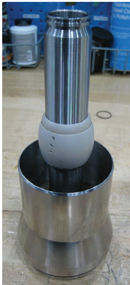
4. Nozzle and lock ring slides over spindle.
