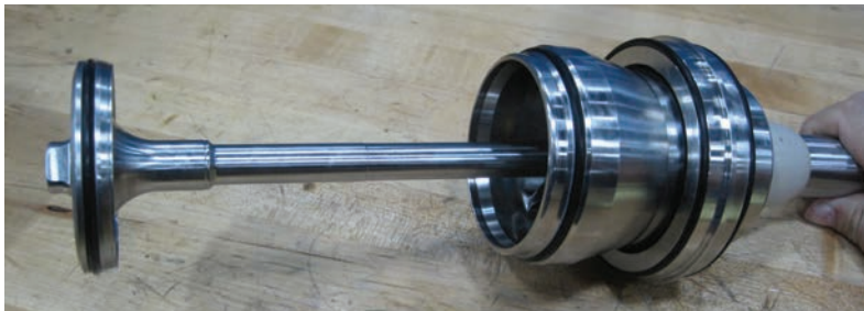
12. Insert tank plug from the bottom of upper plug.
