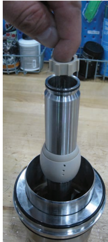
12. Insert tank plug from the bottom of upper plug.
